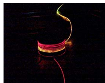
Figure 1. Generation of supercontinuum along a MF.
